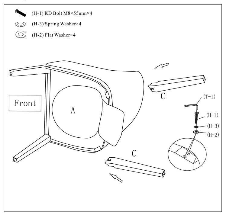
Insert Rear Legs (C) into position. Secure the legs using KD Bolts (H-1), Spring Washers (H-3) and Flat Washers (H-2), stacking the hardware in the order as shown. Fully engage all bolts but do not tighten them until Step 3.
