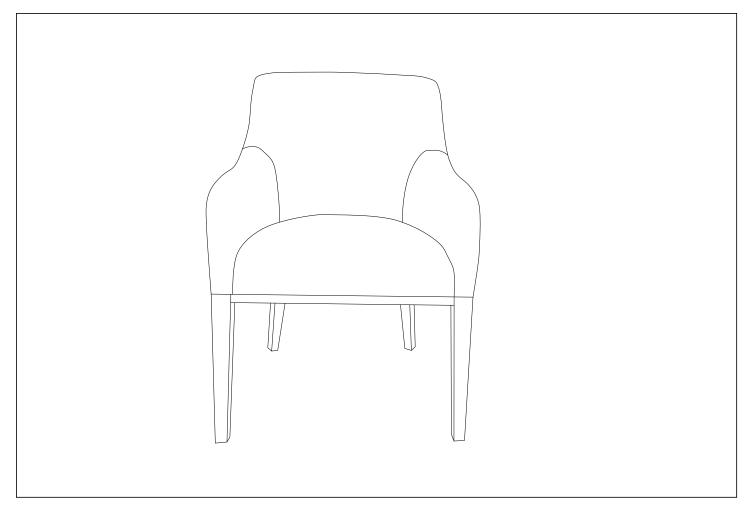
Carefully turn the chair assembly upright and ensure that it rests evenly and level on all four legs. Once level, carefully tilt the chair back down and fully tighten all KD Bolts (H-1) from Steps 1-2 at this time using Allen Wrench (T-1). Zip the cover on the bottom of Seat (A) closed. The chair is now ready for use.
